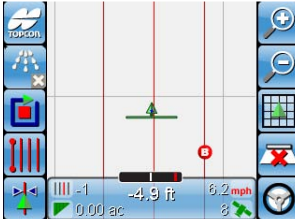
Figure 9-52. Guidance Pattern will load on screen
