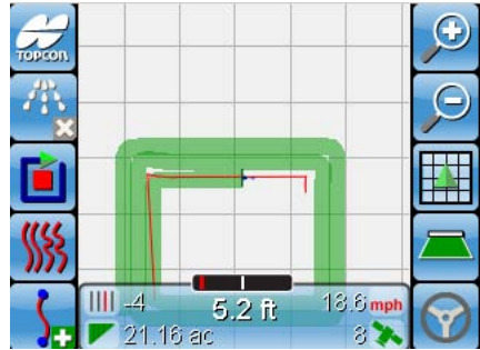
Figure 9-17. New Curve lines will appear based on previous coverage line
