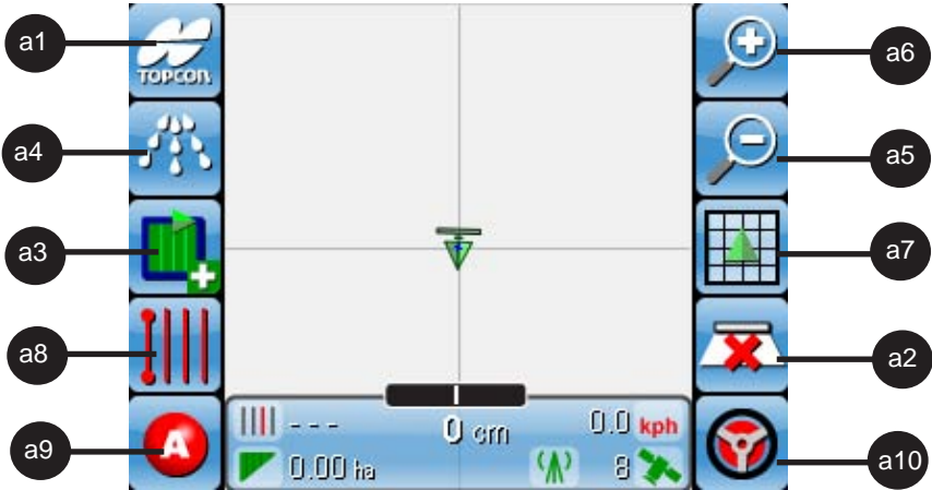
Figure 6-5. Guidance screen with Sprayer and Auto-steer features enabled
