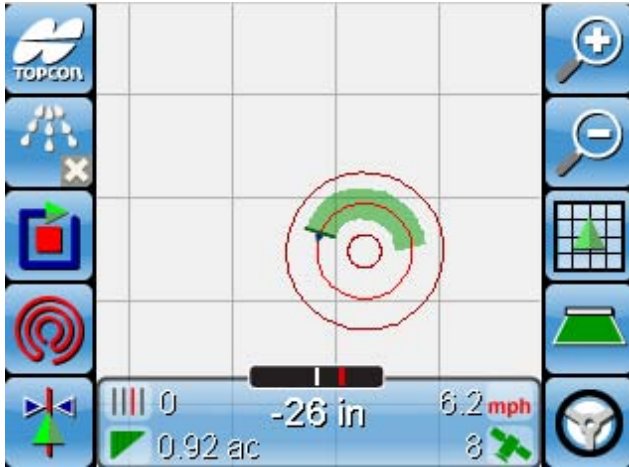
Figure 9-47. A red circle will appear when pivot point is determined
