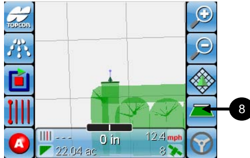
Figure 8-7. Coverage mapping is ON
