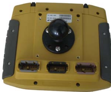
Figure 5-3. Ball Mount Attached to Rear of System 110/150
