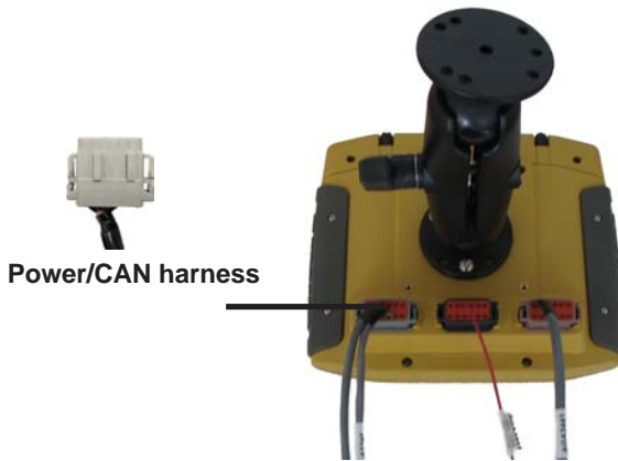
Figure 5-8. Fit Power/CAN harness to Color Coded Connection Port
