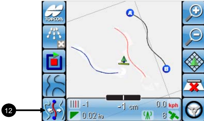
Figure I-13. Select between available Optimal Waylines
