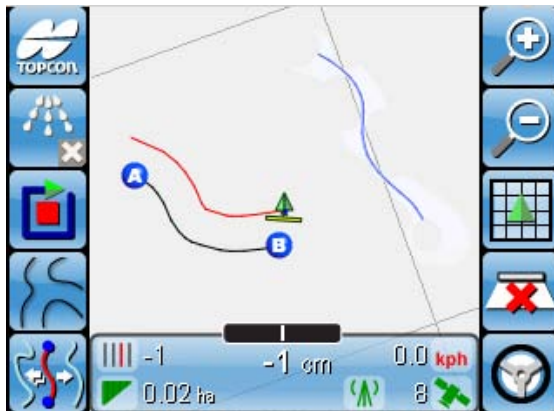
Figure I-12. Optimal Waylines Imported to Console
