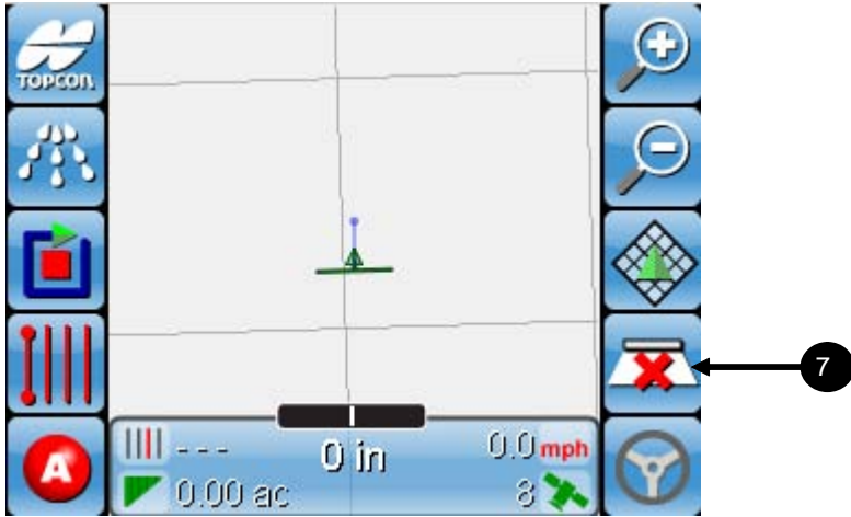
Figure 8-6. Start Coverage Mapping
