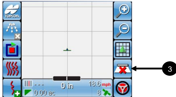
Figure 9-19. Start coverage mapping
