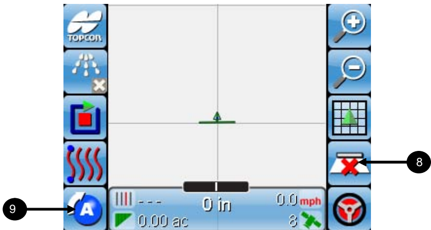
Figure 9-5. Start coverage mapping
