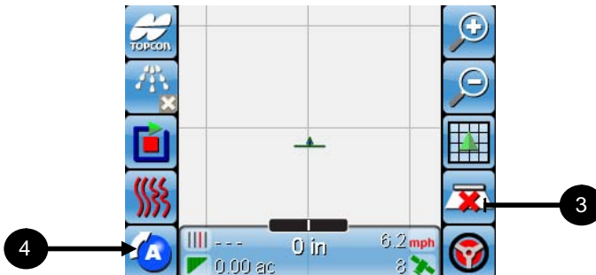
Figure 9-28. Start coverage mapping
