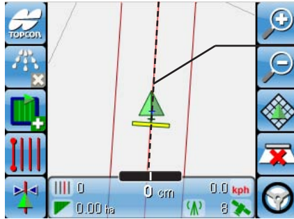
Figure 6-52. GPS Drift Compensation
