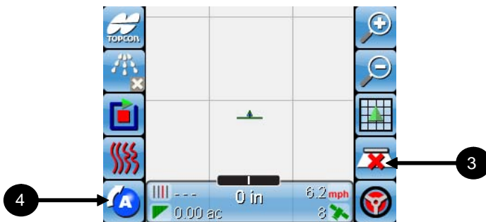
Figure 9-22. Start coverage mapping
