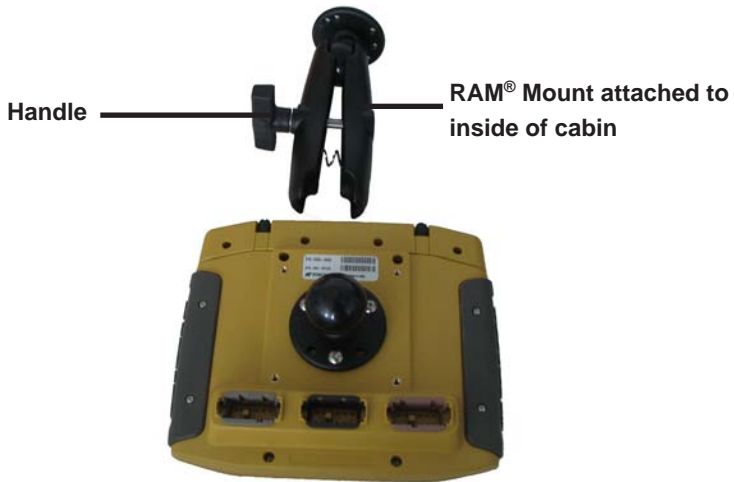
Figure 5-4. Attach the System 110/150 to the RAM® Mount
