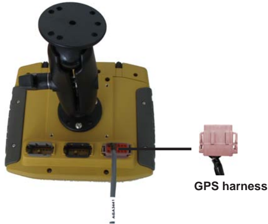
Figure 5-6. Fit GPS Harness to Color Coded Connection Port
