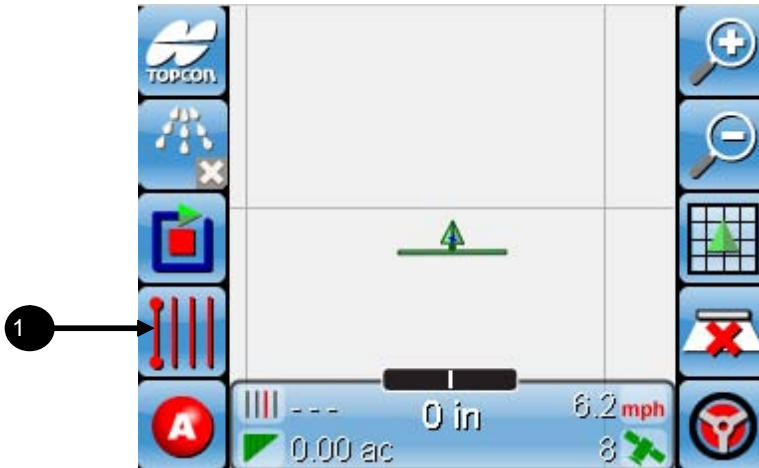
Figure 9-49. Access the Guidance Pattern screen
