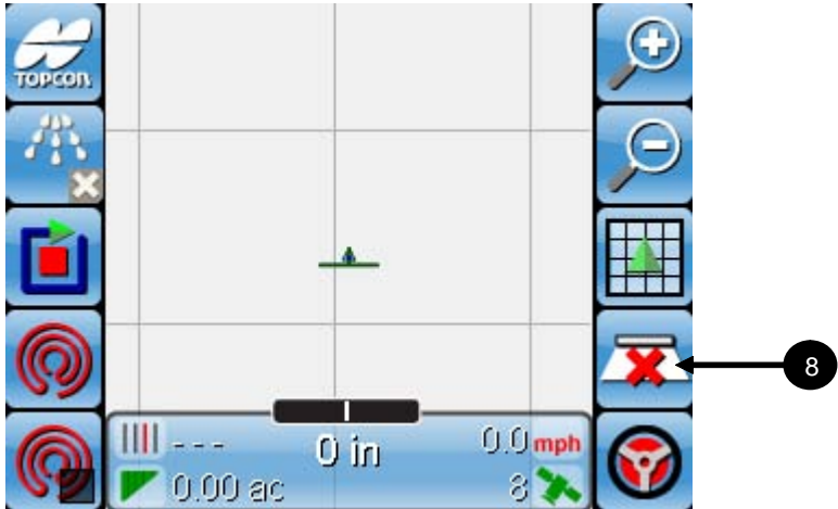
Figure 9-45. Start Coverage mapping
