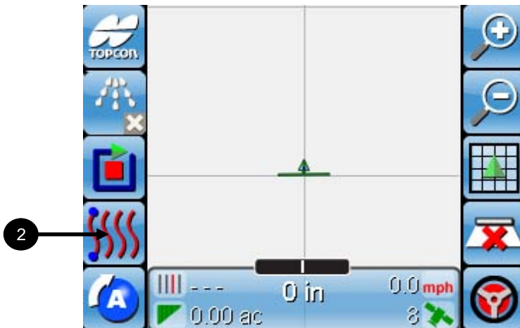
Figure 9-1. Access Guidance Pattern screen
