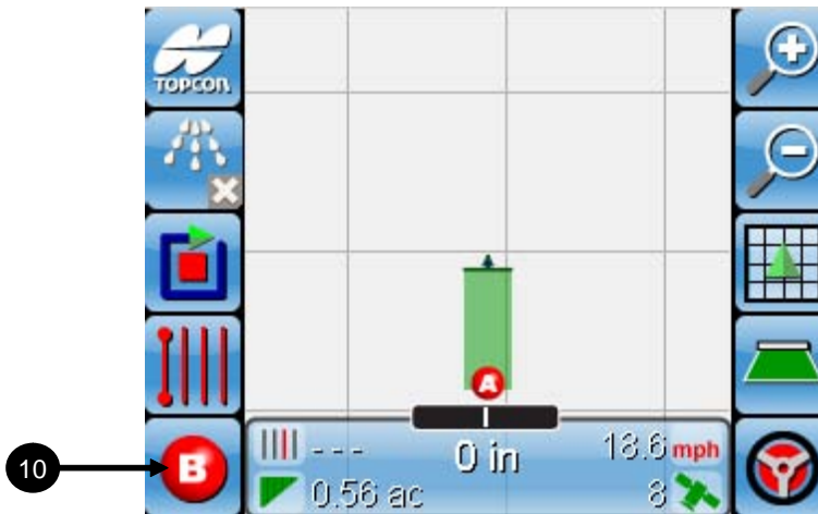
Figure 9-38. Set the first point of the AB line
