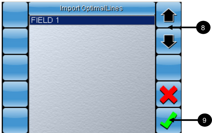
Figure I-10. Import Optimal Waylines screen
