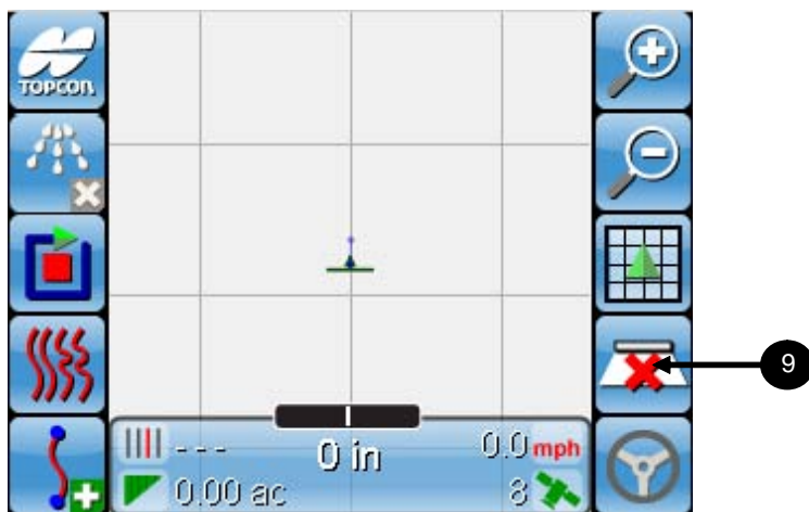
Figure 9-13. Start coverage mapping
