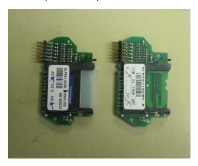
5. Insert the replacement sd card slot into the monitor. Pay special attention to the micro-chip prongs that get inserted into the green circuit board. Gently push the sd card slot into place.
