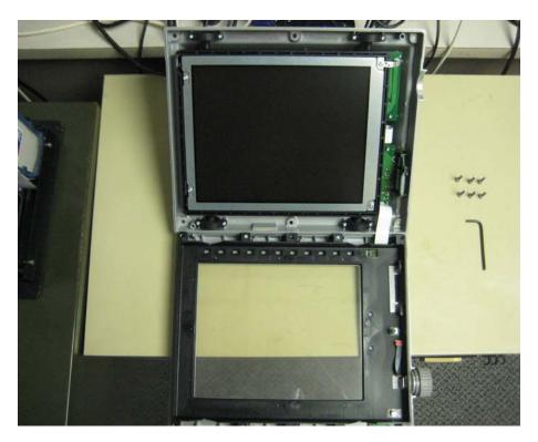
3. Remove the damaged card slot from the monitor.
