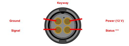
12 volts applied to the Signal wire will open the valve while no voltage on the wire will close it.
