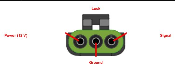
For boom valves, 12 volts on the Signal wire will open the valve while no voltage on the wire will close it.\*
