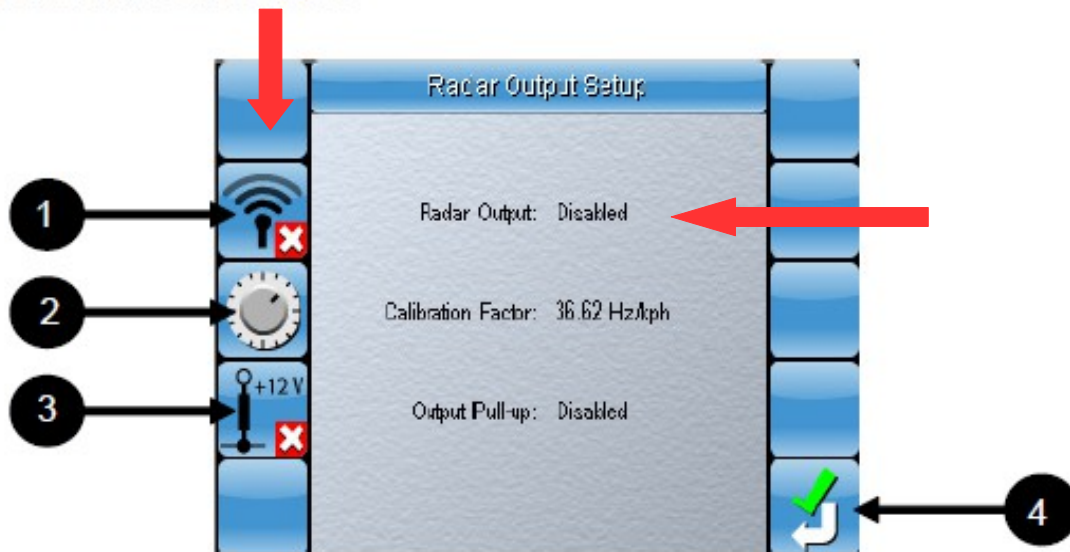
Figure 6-43. Radar Output Setup
